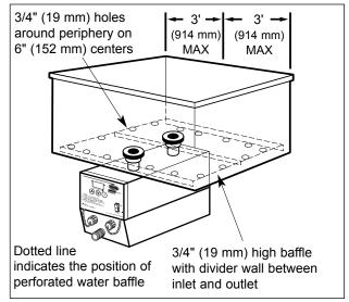
Figure 6. Hydro-Heater Water Baffle
